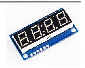
7-segment LED displays are used in many projects to visualize informations; their use is simple as lighting a LED, but it should be complicated because of the need to manage a lot of interface signals to organize more than a digit at the same time, especially when the control device used doesn't provide enough I/O lines.
