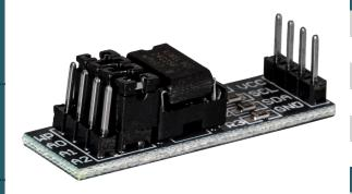
This EEPROM memory allows you to store and read data externally via the I2C interface of your microcontroller.
