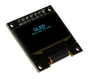
The compact 0.96 inch (approx. 2.44 cm) OLED display is the perfect solution for your projects. Thanks to the flexible control via I2C or SPI, it can be easily integrated with Arduino, Raspberry Pi and other microcontrollers or single-board computers.
